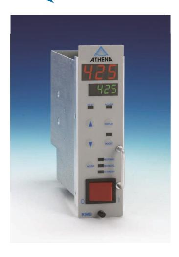
Athena's Series RMB Modular Hot Runner controller is a microprocessor-based, single-zone temperature controller specifically designed for runnerless molding applications. The controller is fully self-tuning, with built-in diagnostics, and features an easy-to-use operator keypad with simultaneous process and set point displays and discrete indicators for heat output, alarm, degrees F/C, manual/closed loop mode, and CompuStep®.
