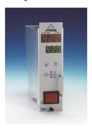
Athena's Series RMA Modular Hot Runner controller is a microprocessor-based, single-zone temperature controller specifically designed for runnerless molding applications. The controller is fully self-tuning, with built-in diagnostics, and features an easy-to-use operator keypad with simultaneous process and set point displays and discrete indicators for heat output, alarm, degrees F/C, manual/closed loop mode, and CompuStep®.
