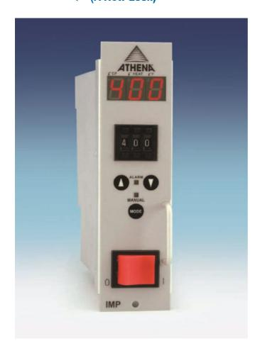
Athena's Series IMP Modular Hot Runner controller is a microprocessor-based, single-zone temperature controller specifically designed for runnerless molding applications. The controller is fully self-tuning, with built-in diagnostics, and features an easy-to-use operator keypad with simultaneous process and set point displays and discrete indicators for heat output, alarm, degrees F/C, manual/closed loop mode, and CompuStep®.
