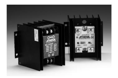
The Athena ZC and PC contactors are available as zero voltage switched (ZC) and phase angle-fired (PC) contactors that can be used for control of resistive heater loads. The controller provides full power rating at 102°F (49°C) ambient temperature, and extends heater life while eliminating thermal shock.
