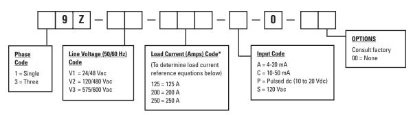
To Order: Determine proper line voltage, load current, input signal and options required, if any.
