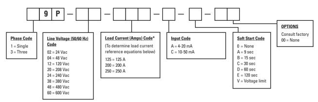
To Order: Determine proper line voltage, load current, and options required, if any.
