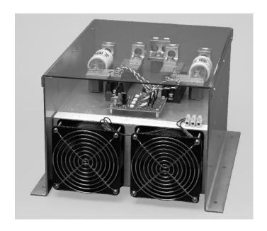
The Athena 19P (single phase) and 39P (three phase) are phase-angle fired power controllers that can be used for control of resistive heater loads. The high amperage series provides capacity from 125 amps up to 250 amps and the controllers are designed to extend heater life while eliminating thermal shock.
