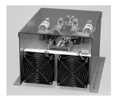
The Athena 19Z (single phase) and 39Z (three phase) are zero switched power controllers that can be used for control of resistive heater loads. The high amperage series provides capacity from 125 amps up to 250 amps. The controllers are designed to extend heater life while eliminating thermal shock.
