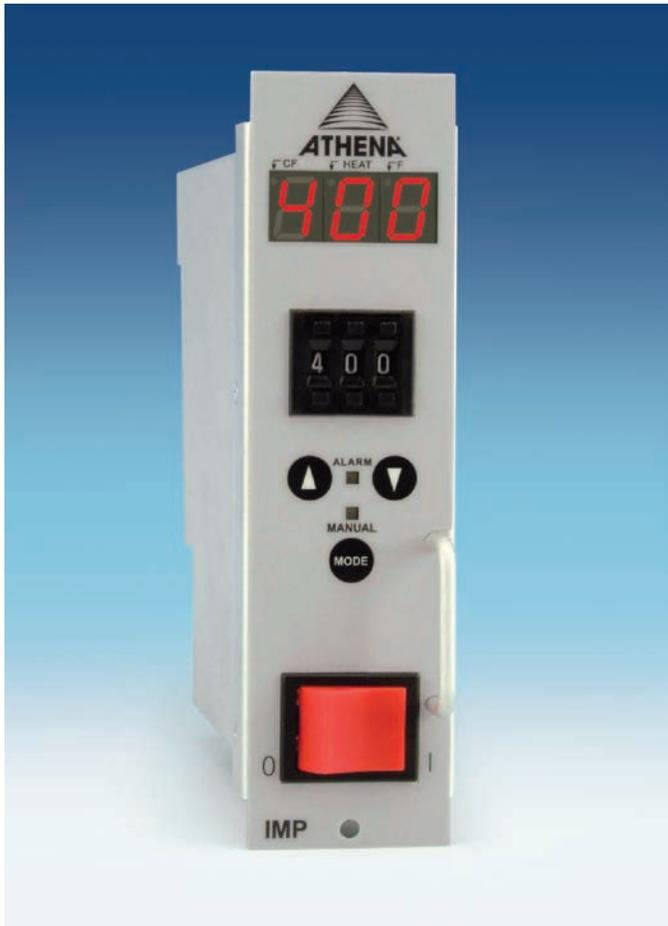
Athena's Series IMP Modular Hot Runner controller is a microprocessor-based, single-zone temperature controller specifically designed for runnerless molding applications. The controller is fully self-tuning, with built-in diagnostics, and features an easy-to-use operator keypad with simultaneous process and set point displays and discrete indicators for heat output, alarm, degrees F/C, manual/closed loop mode, and CompuStep®.
