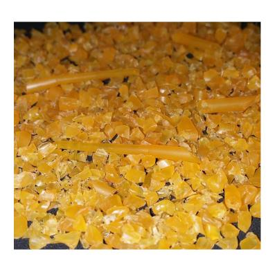
6 mm angular drilled screen
