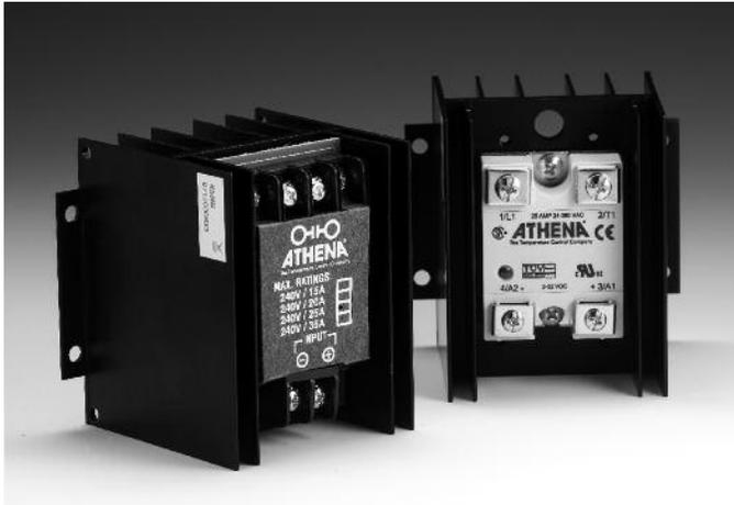
The Athena ZC and PC contactors are available as zero voltage switched (ZC) and phase angle-fired (PC) contactors that can be used for control of resistive heater loads. The controller provides full power rating at 102°F (49°C) ambient temperature, and extends heater life while eliminating thermal shock.
