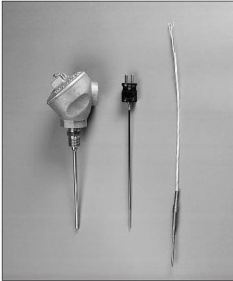
Tu-Pak® is Athena's trademark for metal-sheathed, mineral-insulated (MI) thermocouple material. It is a departure from the traditional assembly of tubes, wires and insulators. It has a unit-construction with no replacement parts. Tu-Pak® has improved thermal response, greater flexibility and, size for size, it is longer lasting than traditional types.
