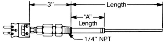
Custom Vacuum Furnace Thermocouple
