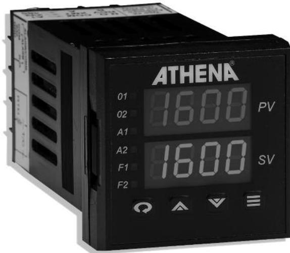
The Athena 16C is a 1/16 DIN panel mounted, auto-tuning controller that can be used for precise control of a single loop with two independent outputs field-configurable as direct acting, reverse acting or alarm. RS-232 or RS-485 communications interfaces are available, and two digital LED displays provide visual indication of various controller functions.
