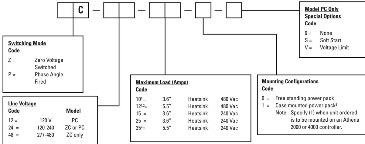
**Example:** Model ZC-2425-1-a controller with a zero voltage switching mode; a line voltage of 120-240 V; a maximum load (amps) of a 3.6" heatsink, 240 Vac; and a case-mounted power pack configuration.
