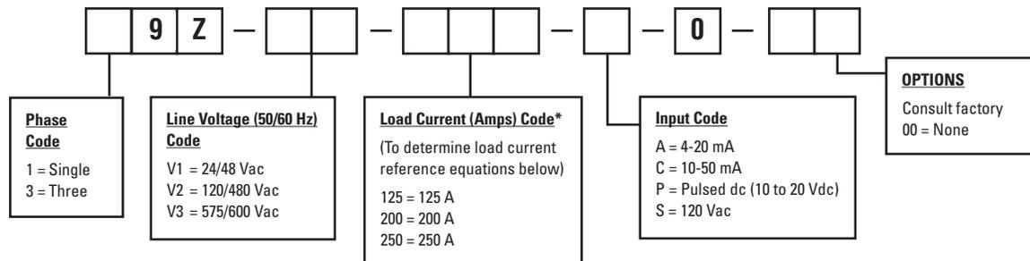
**To Order:** Determine proper line voltage, load current, input signal and options required, if any.
