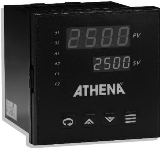
The Athena 25C is a 1/4 DIN panel mounted, auto-tuning controller that can be used for precise control of a single loop with two independent outputs field-configurable as direct acting, reverse acting, and 2 alarms. RS-232 or RS-485 communications interfaces are available, and two digital LED displays provide visual indication of various controller functions.
