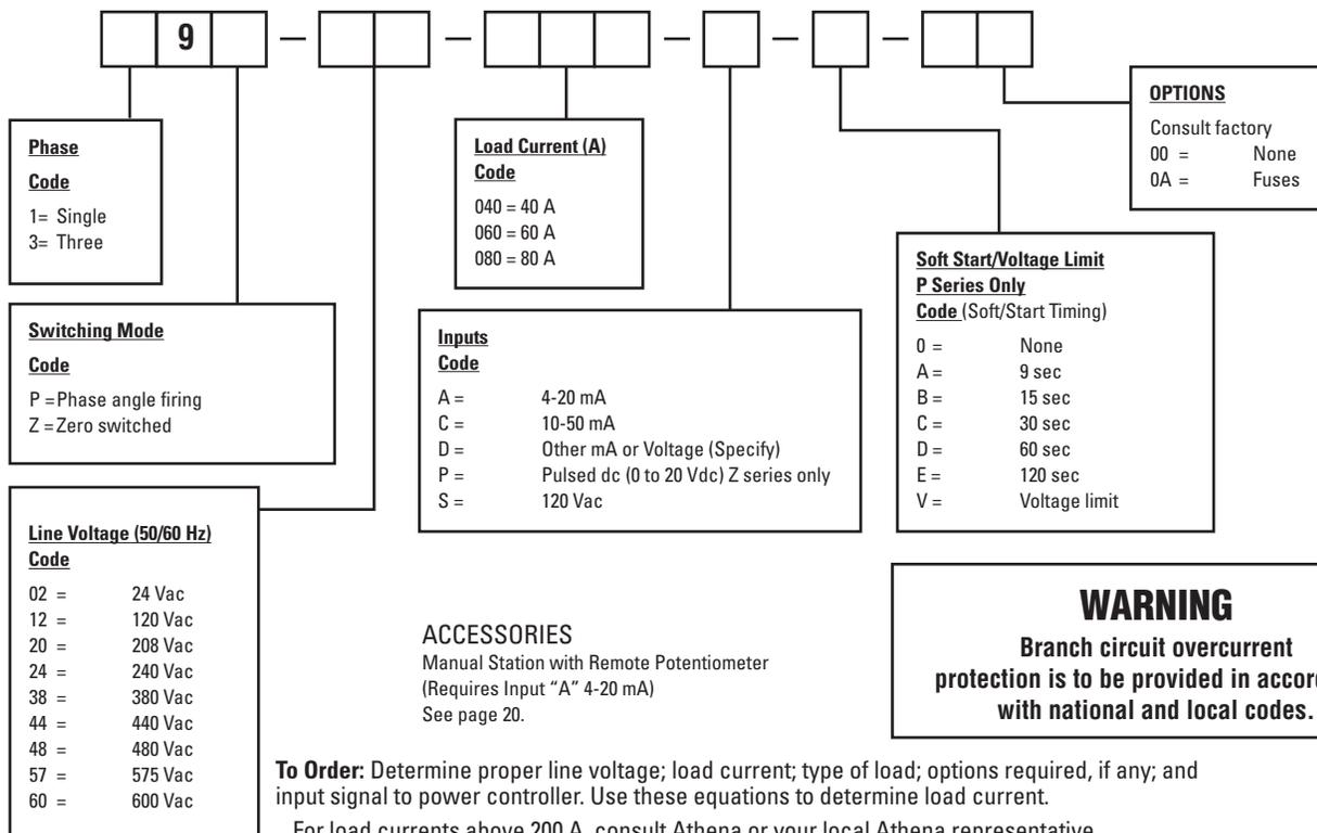
**To Order:** Determine proper line voltage; load current; type of load; options required, if any; and input signal to power controller. Use these equations to determine load current.
