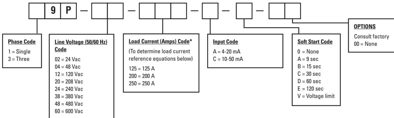
**To Order:** Determine proper line voltage, load current, and options required, if any.
