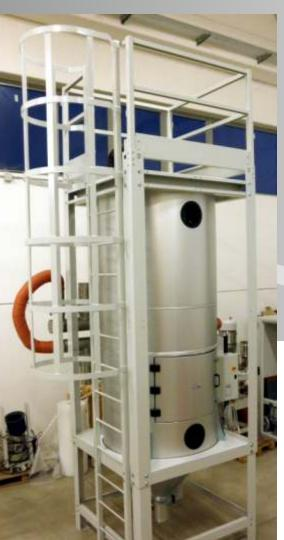
Drying hoppers are fully insulated with individual heaters and temperature setting controls. The cylindrical shape ensures uniform drying.
